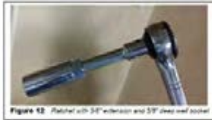
Figure 12 Ratchet with 3/4" extension and 3/8" deep well socket
