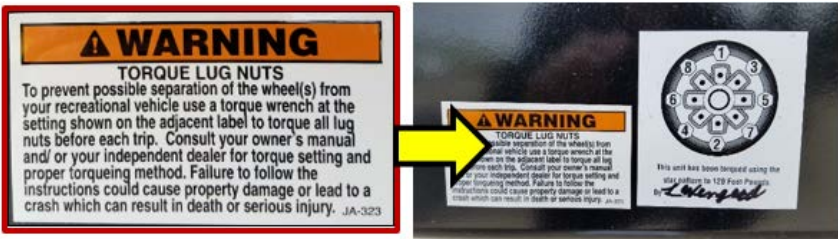
Lug nut torque pattern and warning label
