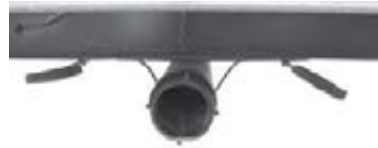
Black/Grey Tank Drain and Valves
