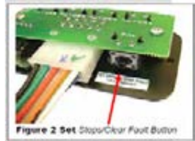
Figure 2 Set Stop-Clear Fault Button
